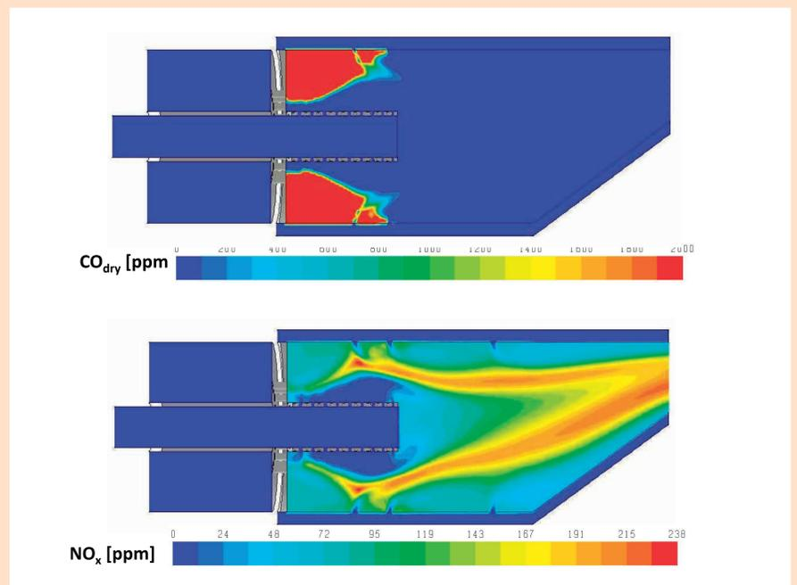
CFD results: Typical field distribution of CO and NO<sub>x</sub> emission values for the new combustor
