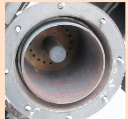
View inside the gas turbine combustor
