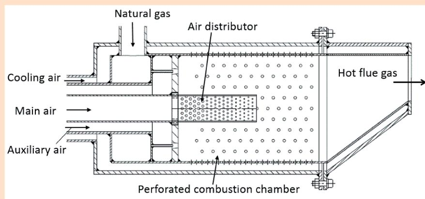
Schematic design of the new gas turbine combustor
