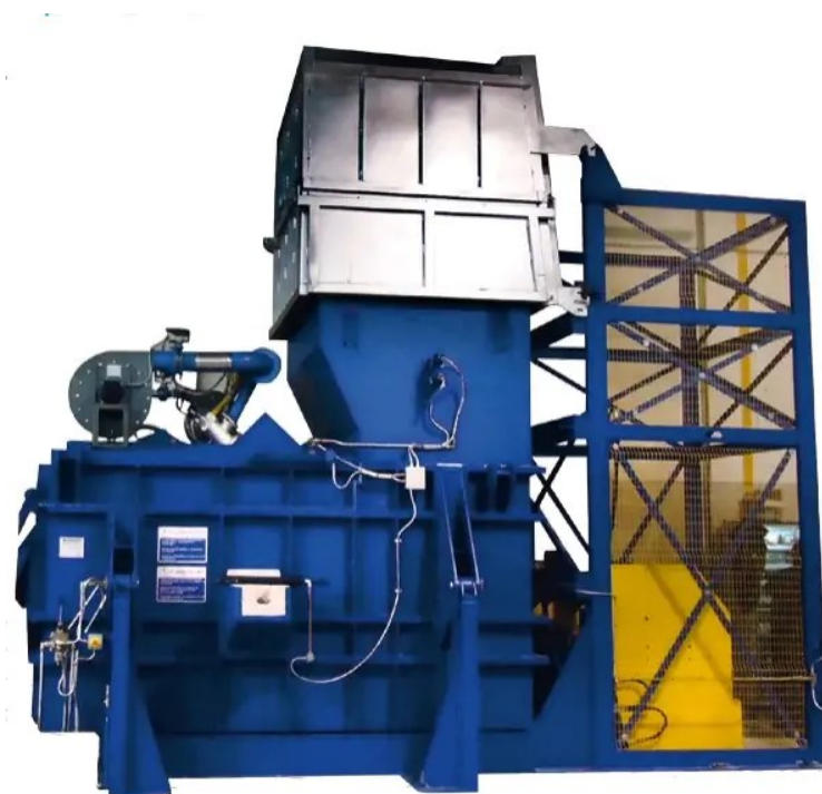
Figure 19: Images of a melting tower for aluminium recycling (Source: MARCONI).
