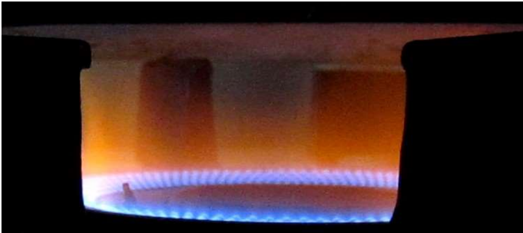
Figure 55: yellow flame on EB15.
