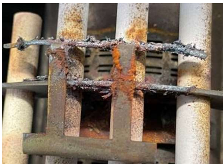
Figure 36: Illustration of flashback effect on GA16, with 40%H2.
