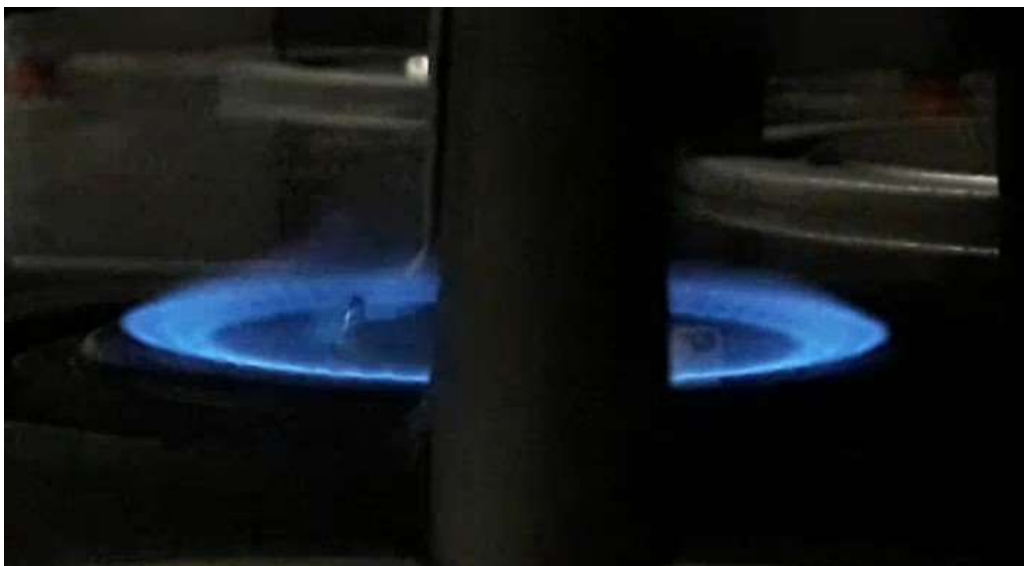
Figure 56: EN12 Burner under "normal" operation.
