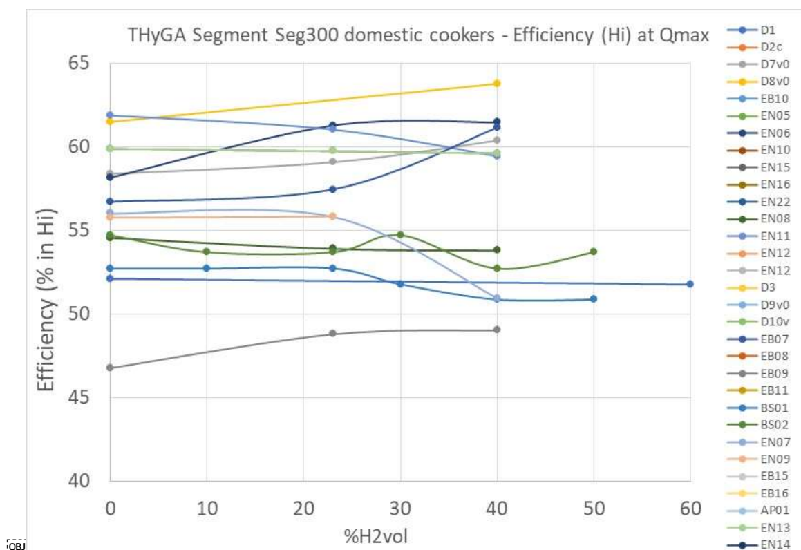
Figure 72: Segment 300 – Efficiency at Qmax (when a curve is missing for an appliance it means it was not measured).
