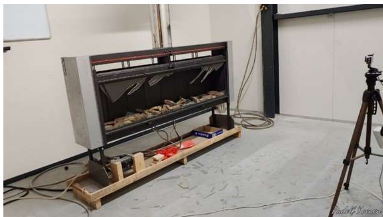
Figure 132: Experimental setting for the delayed ignition test.
