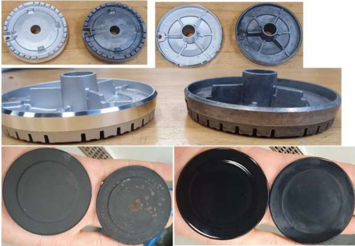
Figure 53: Comparison of parts before/after tests for cooker 1
