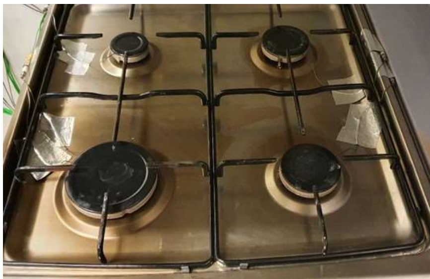
Figure 33: Plates setup above, temperature probes setup underneath
