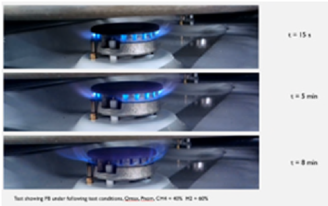
Figure 7: Flashback on a cooking burner (bottom photography)
