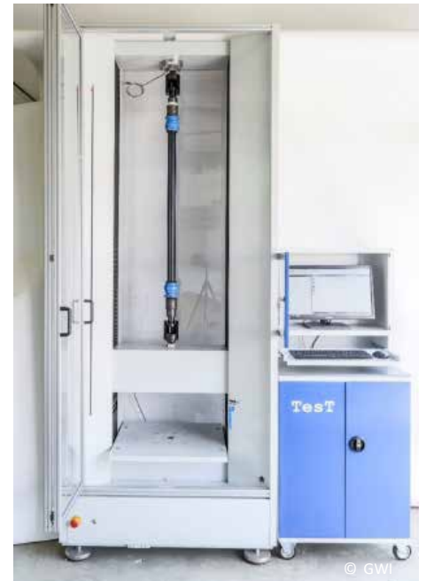
COMPUTER-CONTROLLED TENSILE AND COMPRESSION TESTING MACHINES WITH CAPACITIES OF UP TO 2 / 50 / 250 kN, AND PARTIALLY AUTOMATED COMPRESSION STRENGTH TESTING UP TO 500 kN
