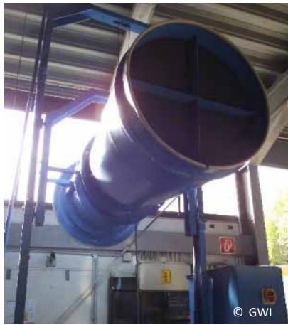
WIND GENERATOR WITH WIND SPEEDS UP TO 15 M/S
