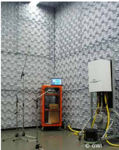
ACOUSTIC TESTING ACCORDING TO DIN EN 15036
