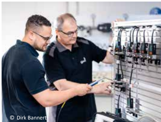
TEST BENCH FOR LEAK RATE DETERMINATION
