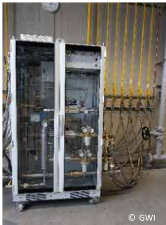
GAS MIXING SYSTEMS UP TO 500 kW RATED CAPACITY WITH NATURAL GAS / GAS MIXTURES
