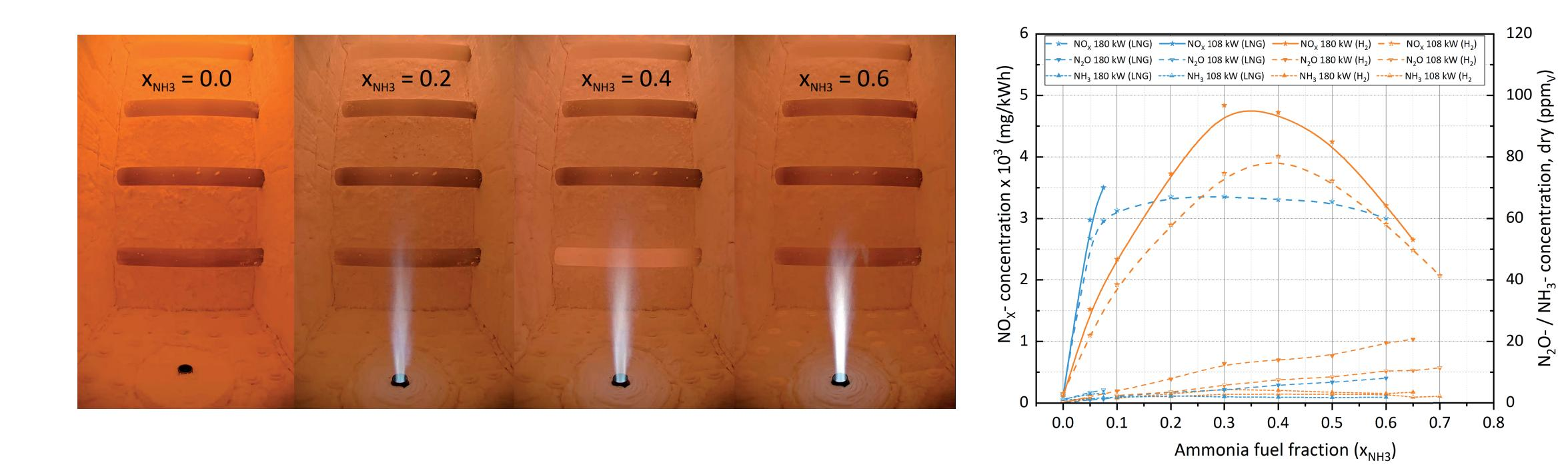
INITIAL STUDIES WITH AN INDUSTRIAL BURNER TO DETERMINE THE MAXIMUM NH<sub>3</sub> ADMIXTURE RATE IN COMBINATION WITH H<sub>2</sub> AND LNG
